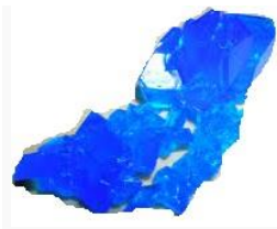
Crystal of copper Sulfate obtained by the crystallization of Copper Sulfate solution
